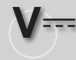
Direct Current V DC All battery operated machines / also used to drive AC powered machines.
