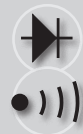
Continuity Check Used to inspect fuses and circuitry. A beep will sound when fuse or circuit is closed.
